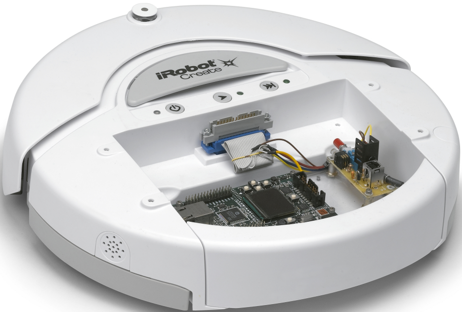
Figure 1.15: iRobot Create with an external microcontroller.
